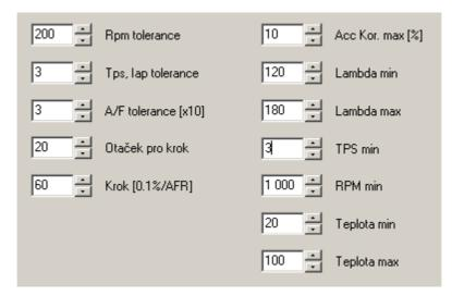
**RPM tolerance** - if engine rotates are away from active rotates column more than in our case 200 RPM the "autotuning" won't work. This limitation applies only for way of tuning "in points".
