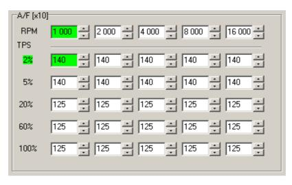
There are map of "Request of AFR" at right side of tab-sheet. Value of AFR is multiplied by x 10. Actual AFR request is calculated from actual revolution and throttle position (next only TPS). There is implemented an interpolation between particular points. Example: actual request AFR 14.0 (14kg of air on 1kg fuel) is represent by number 140 in the tab on above mentioned example.
